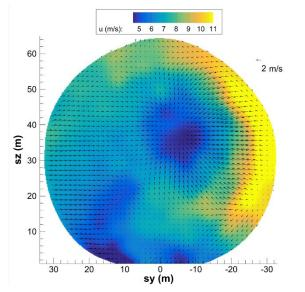
Fig. 2: Example of a 3D reconstructed wind field in the wake of a SWiFT site V27 turbine at 2.5 D downwind. The 3D wind field is reconstructed in less than one second on a PC from 800 sequential line-of-sight radial wind speed measurements scanned by the lidar during a 2 second sampling period. The axial wind component u(y, z) is color coded while the two transverse wind components are represented by black arrows.
