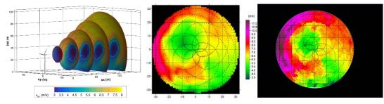
Fig.1. [Left]: SpinnerLidar scanning pattern in the wake of the V27 test turbine at the SWiFT site, overlaid on interpolated lineof-sight speed measurements; [Middle]: Line-of-sight wind speeds measured by the SpinnerLidar on Dec 15<sup>th</sup> 2016 20:31:00 to 20:31:02 at 66.2 m downwind distance, interpolated on a  $1 \times 1$  m grid facing the turbine, i.e. the turbine is behind the frame. [Right]: The corresponding Lincom reconstructed axial wind component, u(y, z).
