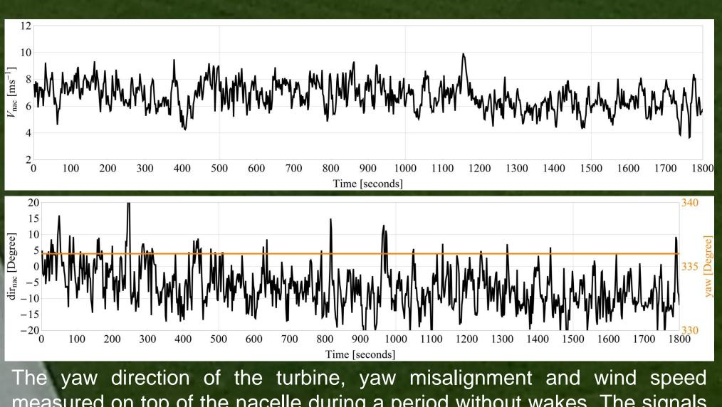
measured on top of the nacelle during a period without wakes. The signals are down-sampled to 0.5 Hz.
