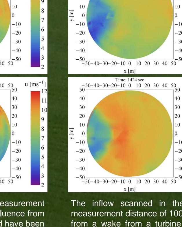
The inflow scanned in the afternoon on a spherical surface at a measurement distance of 100 m during periods of 2 seconds with influence from a wake from a turbine nearby. The line-of-sight speeds measured have been converted to axial (along the rotation axis of the wind turbine rotor) wind speeds corresponding to the measured projection along the line-of-sight of the lidar.
