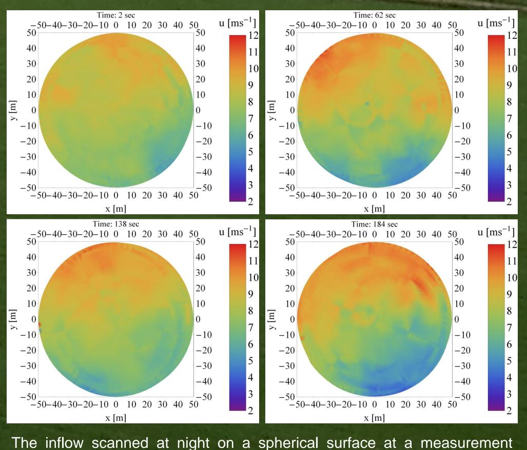
distance of 100 m during periods of 10 seconds without any influence from wakes from nearby turbines. The line-of-sight speeds measured have been converted to axial (along the rotation axis of the wind turbine rotor) wind speeds corresponding to the measured projection along the line-of-sight of the lidar.
