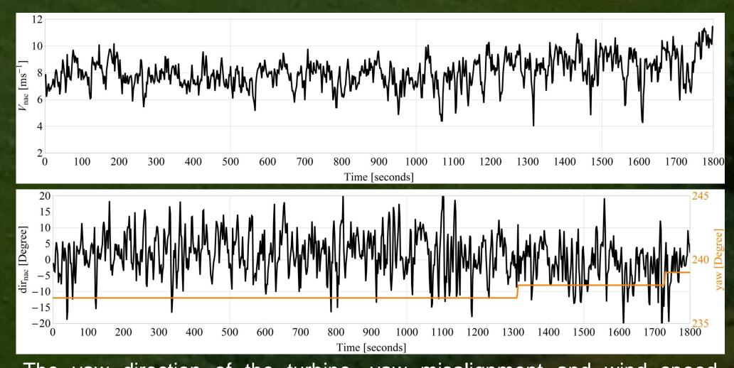
The yaw direction of the turbine, yaw misalignment and wind speed measured on top of the nacelle during a period with wake influence. The signals are down-sampled to 0.5 Hz.
