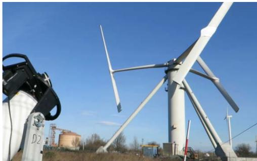
Figure 3. Short range WindScanner R2D2 on operation at the Nenuphar vertical axis offshore prototype, Fos-sur-Mer, Fr.
