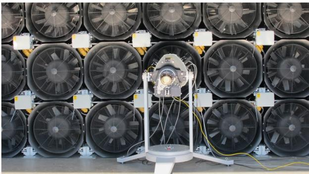
**Figure 6 Short-range WindScanner v1.2 in WindEEE Wind Dome, Canada**
