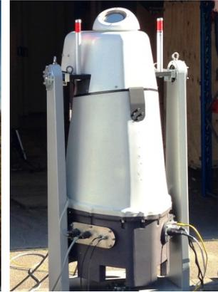
Figure 2 Left: First Short-range WindScanner at DTU Risø Workshop 2010; Middle: Inaugurating the first of three Short-range WindScanners, R2D1 vers. 1.0, Risø DTU 2011; Right: Improved Short-range WindScanner vers. 1.2 Sep 2014).
