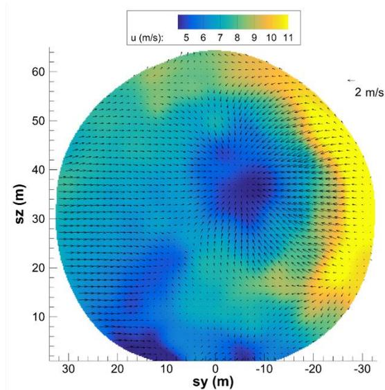
Fig. 2: Example of a 3D reconstructed wind field in the wake of a SWiFT site V27 turbine at 2.5 D downwind. The 3D wind field is reconstructed in less than one second on a PC from 800 sequential line-of-sight radial wind speed measurements scanned by the lidar during a 2 second sampling period. The axial wind component  $u(y, z)$  is color coded while the two transverse wind components are represented by black arrows.
