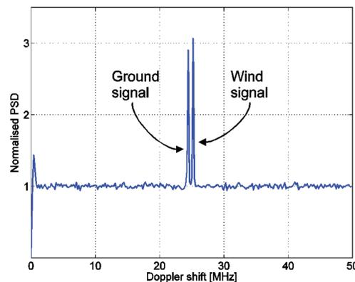
Figure 1. Example of a normalised Doppler spectrum obtained by telescope  $T_1$ . The spectrum is seen to contain two distinct peaks located at 24.4 MHz and 25.2 MHz, respectively. The first peak is due to reflections from the ground when the telescope is pointing downwards and if not filtered out this can lead to erroneous wind speed estimations. The second peak is the wind signal which is the combined effect of the wind and the motion of the blade.
