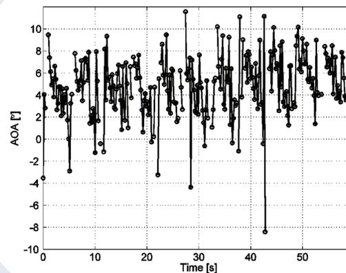
Figure 3. Angle-of-attack (AOA) calculated from the speed measurements shown above. In the beginning of the time series the AOA oscillates around 5 and increases to around 7 in the end. An oscillation with the same frequency as above can be seen, although also some noise is present. Missing data points are seen to appear where the ground signal filter has removed the wind signal from telescope  $T_2$ . This highlights the importance of high data availability.
