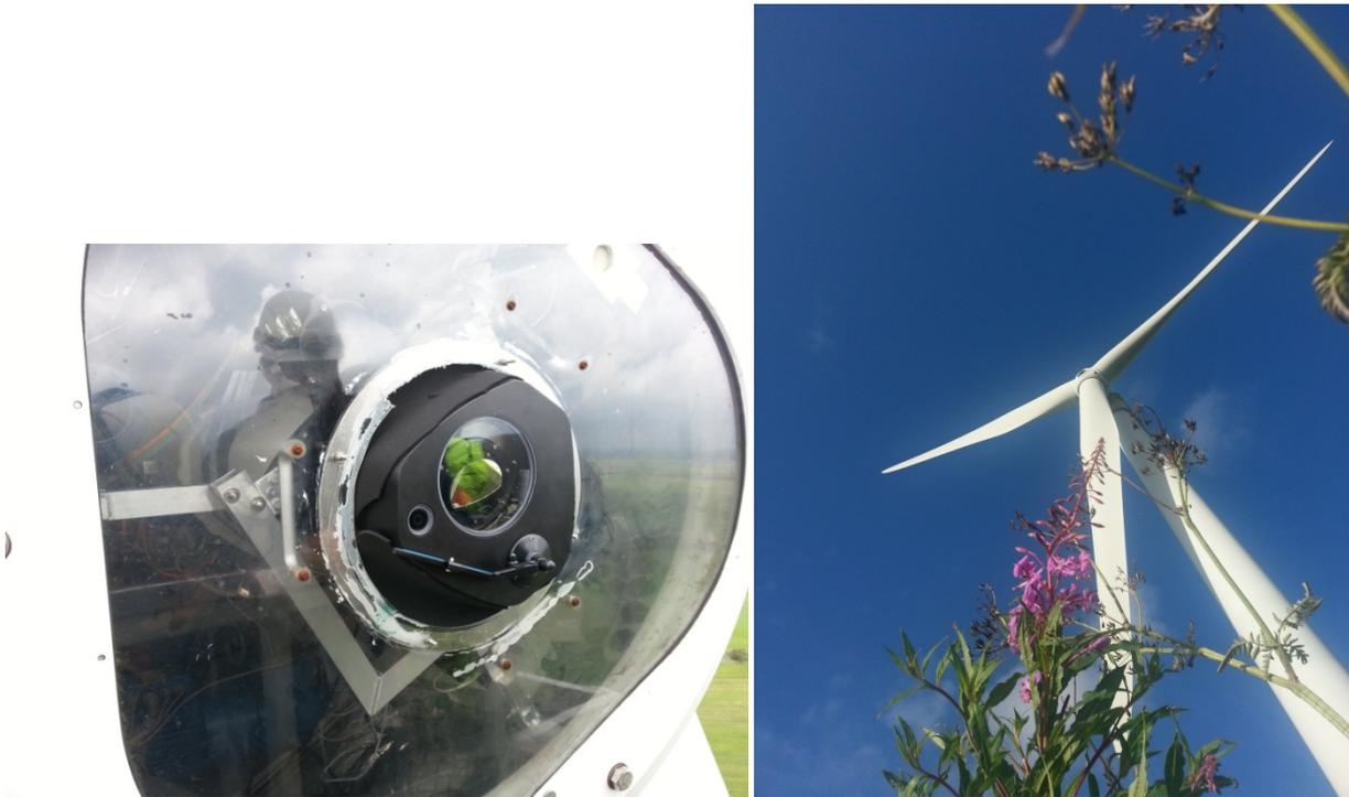
**Figure 11. Left: SpinnerLidar during installation in Dong Energy's NM80 Test Turbine at Tjæreborg Enge (July 2012) Right: NM80 2.3 MW Test Turbine at Tjæreborg Enge, Jutland, Denmark owned by Dong Energy.**
