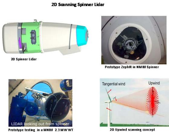
WindScanner Design and Innovation Process: Spinner Lidar and Blade-integrated Lidar's (LIDIC's)
