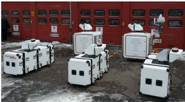
Figur 5. Front row: DTU Wind Energy's set of three own-built prototype Long-Range WindScanners. Second row: Two Long-range WindScanners WLS200S commercially available from Leosphere, Fr
