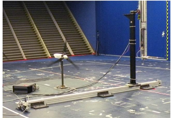
**Figure 9.** The traversing system for the hot-wire probes.
