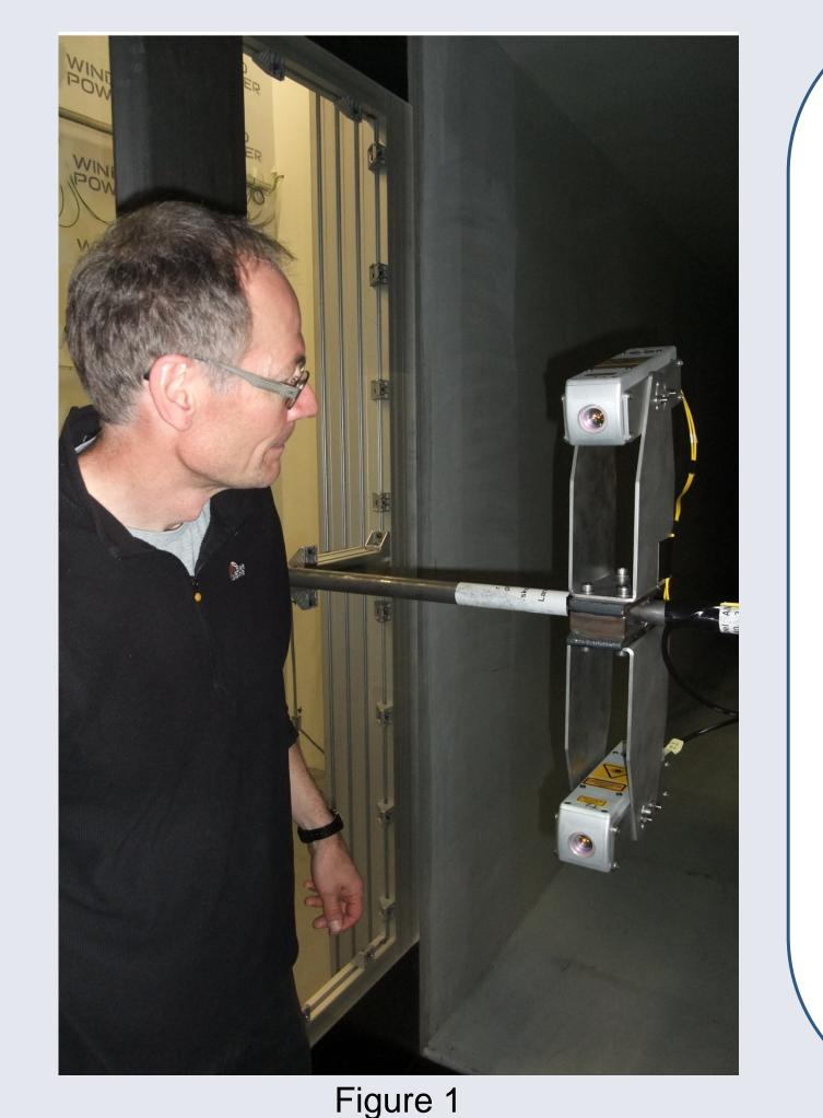
The lidar used is a ZephIR 300<sup>4</sup> with modified transceiver unit, consisting of a telescope with two-inch diameter lens and manually adjustable focus. The telescope is connected to the lidar base unit through fibre optic cables fed through a hole in the tunnel wall, and the base unit is thus placed outside the wind tunnel during operation. The focus of the telescope can be set from 1m to 20m and this short range is necessary due to the tight confinement of the tunnel.
