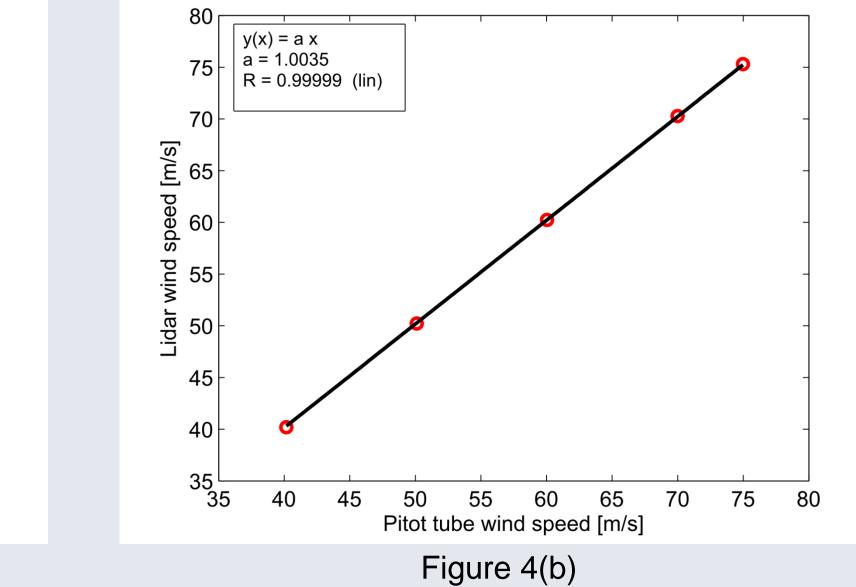
Figures 3(a) and 4(a) show the wind speed measured using the lidar and the two reference systems as function of time. Each step represents two minutes with the wind tunnel running at a constant speed. Figures 3(b) and 4(b) shows the measured mean wind speed over each stable two minute period plotted against the measurements of the reference Pitot tube. Shown is also a linear fit and very good correlation is found in both regimes.
