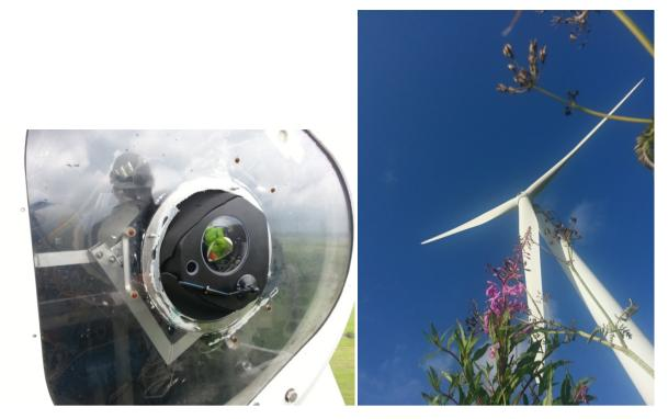
Figure 11. Left: SpinnerLidar during installation in Dong Energy's NM80 Test Turbine at Tjæreborg Enge (July 2012) Right: NM80 2.3 MW Test Turbine at Tjæreborg Enge, Jutland, Denmark owned by Dong Energy.
