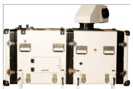
Figure 4. Long-range WindScanner (build from Leosphere WLS200 and equipped with a full-sky  $(2\pi \text{ Sr})$  - DTU Wind Energy – IPU- Leosphere jointly developed two-axis mirror-based scan head.
