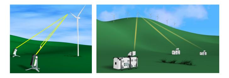
Figure 5. 3D Short-range (10-300 m) wind vector WindScanners at work (concept) Figure 6. 3D Long-range (0.1-10 km) wind vector WindScanners at work (Concept)
