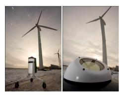
Figure 3. Left: Short-range prism-based half-sky (π Sr) scanhead jointly developed by DTU Wind Energy IPU - Natural Power. Right: WindScanner R2D1.
