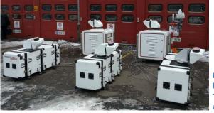
Figur 5. Front row: DTU Wind Energy's set of three ownbuilt prototype Long-Range WindScanners. Second row: Two Long-range WindScanners WLS200S commercially available from Leosphere, Fr
