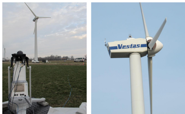
FIG. 3. Lidar 2 positioned in the field with V27 wind turbine in the background (left). Close-up of V27 nacelle and rotor (right).
