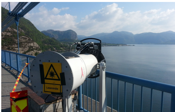
Fig. 9. Short-range WindScanner deployed from the bridge walkaway.
